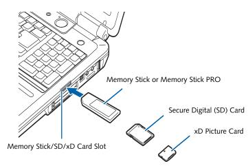
Figure 4-1. Inserting a Memory Stick/SD/xD Card
